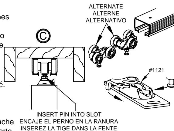
**10** Install finished jambs, split header and casing as shown. Fasten split header on 1121 lock lever side with screws for future door removal or adjustment. **DO NOT USE JAMBS WITH DADO'S.**
