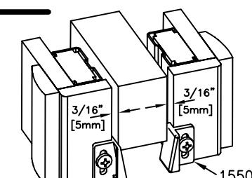
**Fasten** 1550 Guides on finished split jambs at door bottom so door is held in center of opening.
